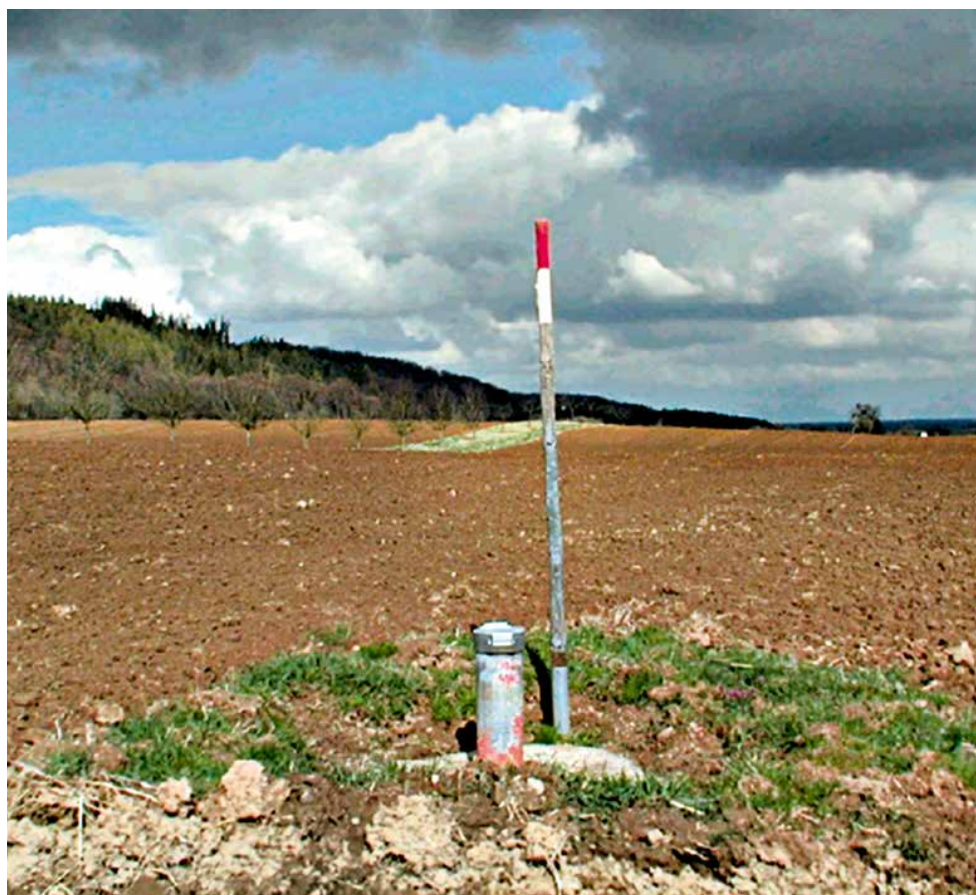
At groundwater measurement points, water resources are continually monitored and the composition of the groundwater is tested.
