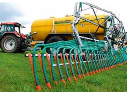
Hose dispensers enable farmers to apply just the necessary amounts of liquid manure fertiliser in a precise manner. This not only reduces the offensive odours, but also prevents excess concentrations of nitrates in the soil.
