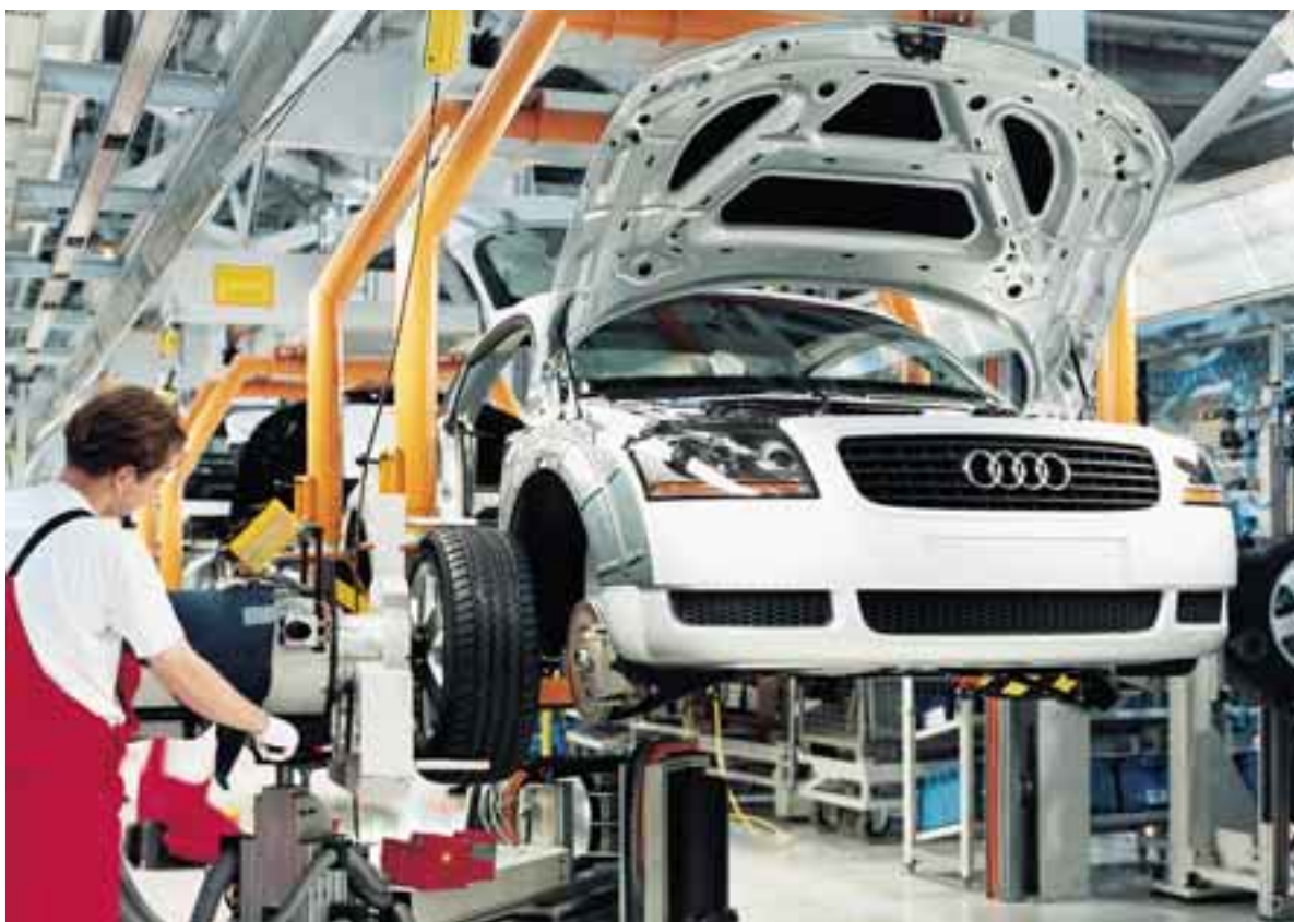
The final production stage involves the fitting of wheels, seats and shock absorbers.
