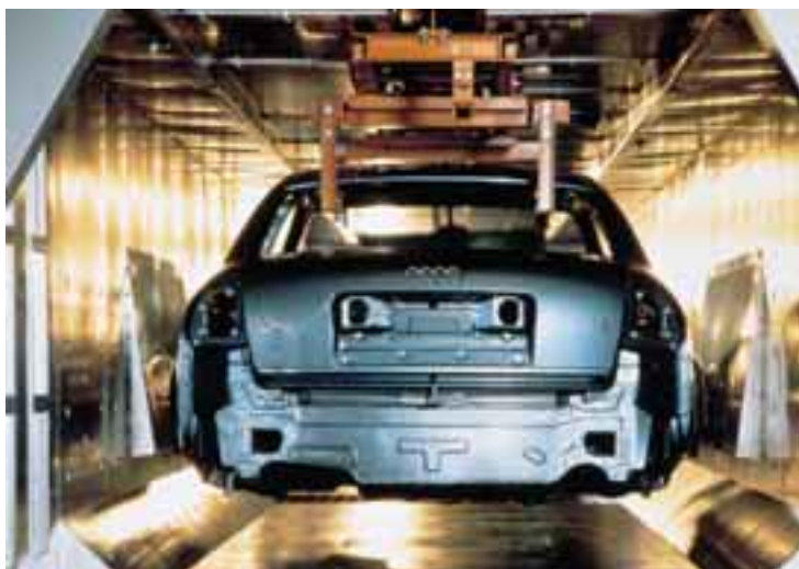
In the paint shop, the car body is preheated in preparation for the hot-flooding process.
