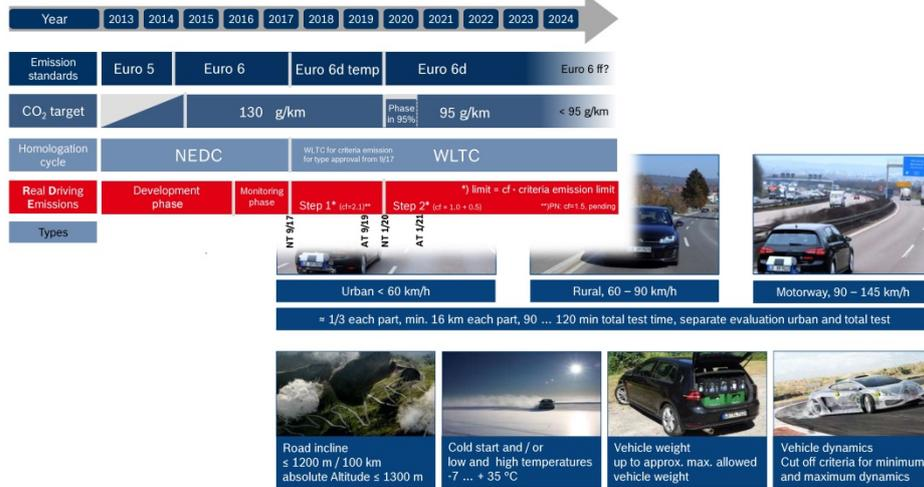
Extreme wide range of possible operation conditions for RDE testing must be covered
