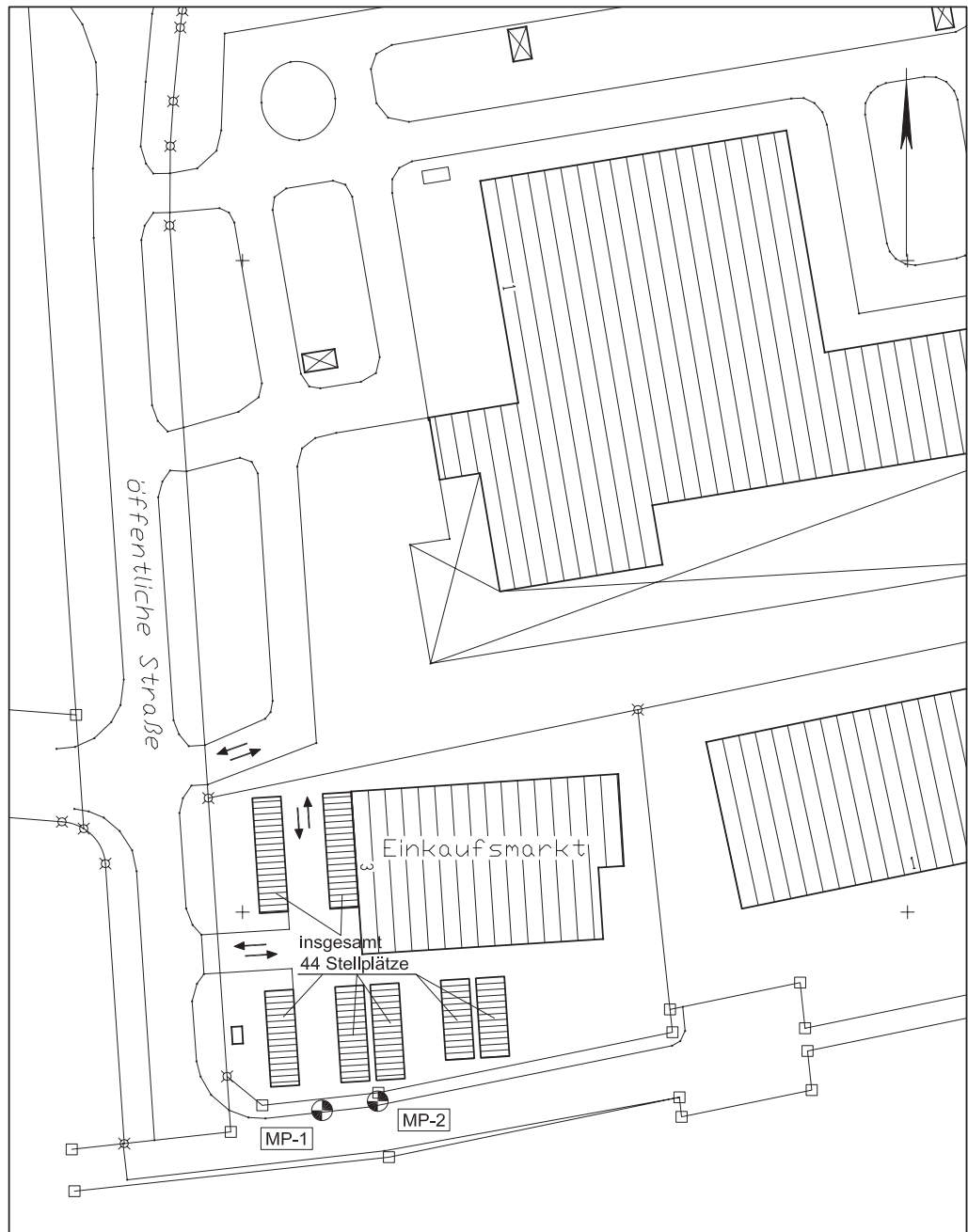
Fig. 33: Site plan of the controlling measurements near a purchase market, measuring points (MP) 3 m above ground (with use of the base data of the Bavarian Measurement Administration; reproduction of the cadastral map M = 1: 1000 by approval of the Bavarian Land Surveying Office München Nr. 1442/03)
