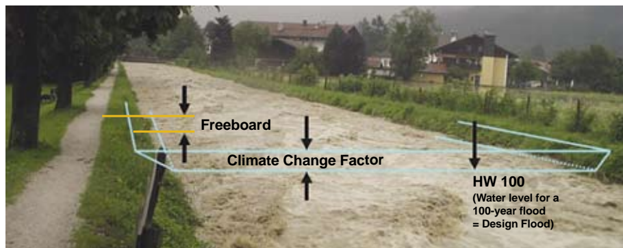
The climate change factor is added onto the one-hundred year flood discharge, resulting in a design flood on which protection measures are based, thereby taking climate change into account.
