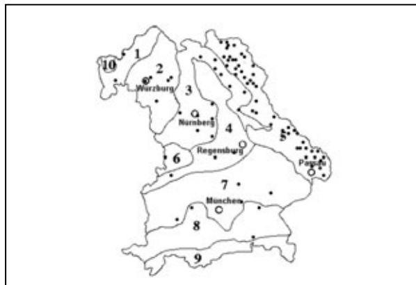
Figure 1 – the ten main regions of Bavaria within which the same geogenic radon potential can be expected. The regions with the highest geogenic radon potential are regions 5 and 10. Rock types of the regions: new red sandstone (1); shell limestone, Keuper (2); Franconian Keuper (3); Upper Jurassic, Dogger, Cretaceous (4); Granite, Gneiss (5, 10); Ejection material of the Ries meteorite (6); Sediment rocks, Molasses (7); young moraine (8); Trias, Jura, Tertiary (9). The dots show the location of all 79 water supply facilities with initial personnel exposure levels exceeding the action level of 6 mSv/a.
