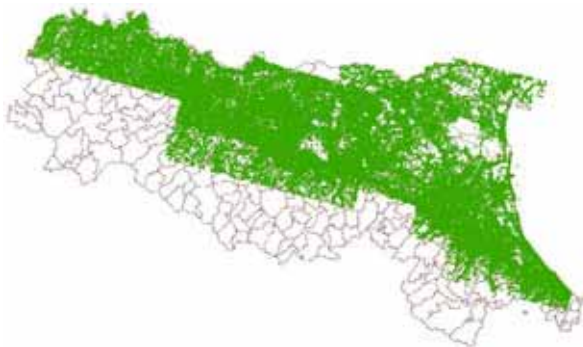
Figure 3: PS coverage of the Emilia Romagna plain using more than 500 radar scenes.
