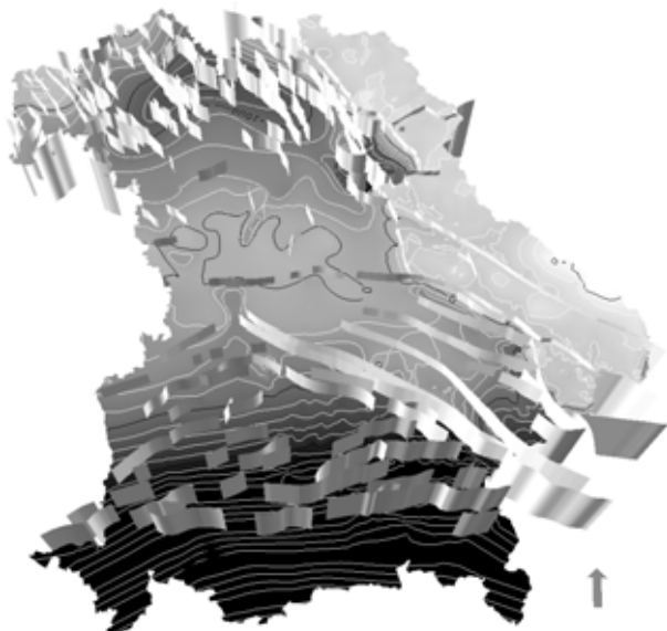
Figure 2 – The non-faulted basement surface with a preliminary simplified fault network.
