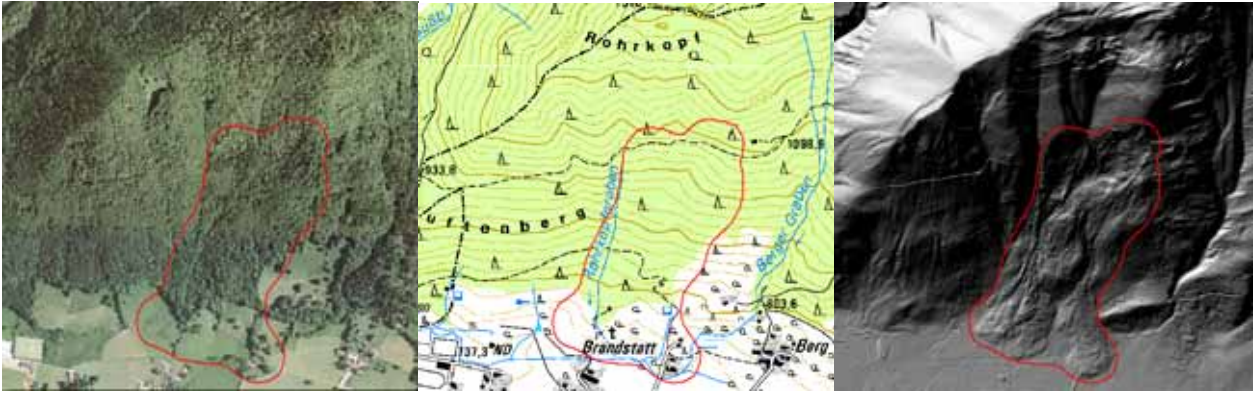
Figure 1 – Areal photographs, topographic maps and HR DEMs in comparison, illustrate the high potential of HR DEMs in landslide mapping.
