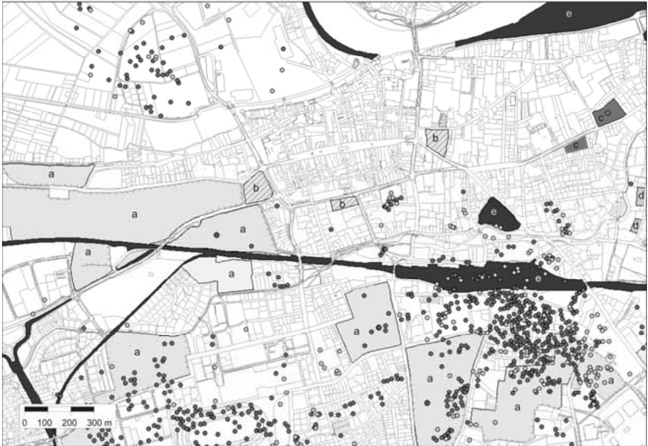
Figure 3 – Anthropogenic overprint in the form of open loam pits (a), completely filled loam pits (b), gravel pits (c), assumed gravel pits (d), land fills (e) and refilled bomb impacts of World War II (circles) in the centre of Straubing.
