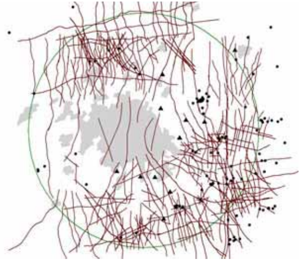
Figure 1 – Working area (circle) around Munich with seismic lines, drillholes from petroleum exploration (dots) and from geothermal drilling (triangles).
