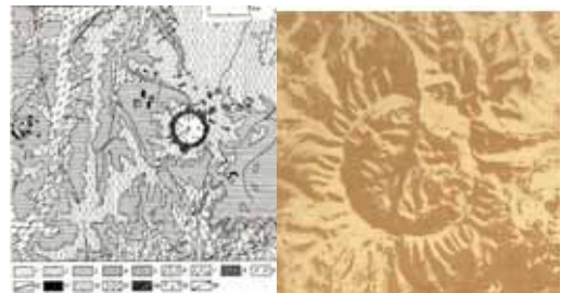
Fig. 8. Geological map (a) and aerial image (b) of Kondyor massif area: 1-3 – Upper PR; 4-5 – Lower PR; 6-8 – AR; 9 – granite, diorite (AR); 10 – diabase (D 2 ); 11-14 – granitoids (J-K); 15 – dunite, pyroxenite, gabbro, diorite, syenite, pegmatite (Lower MZ), 16 – fault (Nekrasov et al., 1994).
