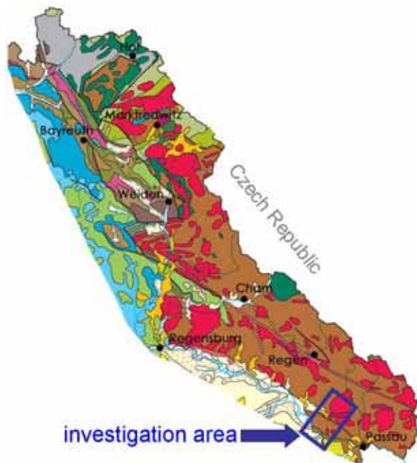
Figure 1 – Target area of the integrated geoscientific mapping project - geological map of East Bavaria with the investigation area for airborne geophysics near Vilshofen (blue rectangle).
