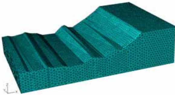
Figure 3 – FE-model for a segment of the slopes in the Isar valley
