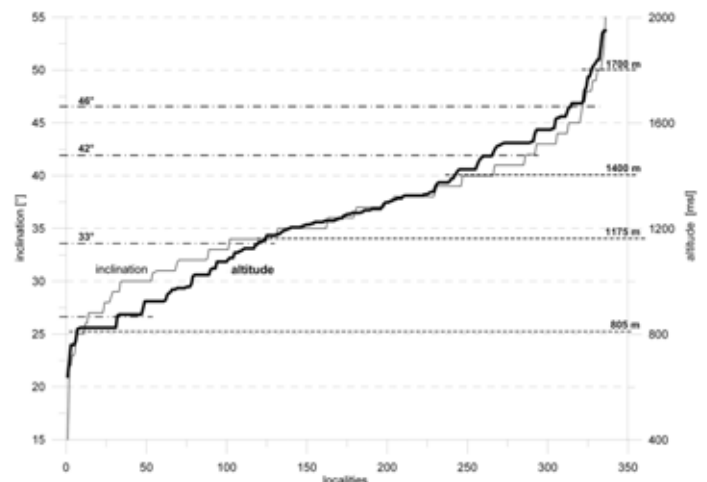
Figure 4 – Separate plots of inclination and altitude, divided into sections of different gradients
