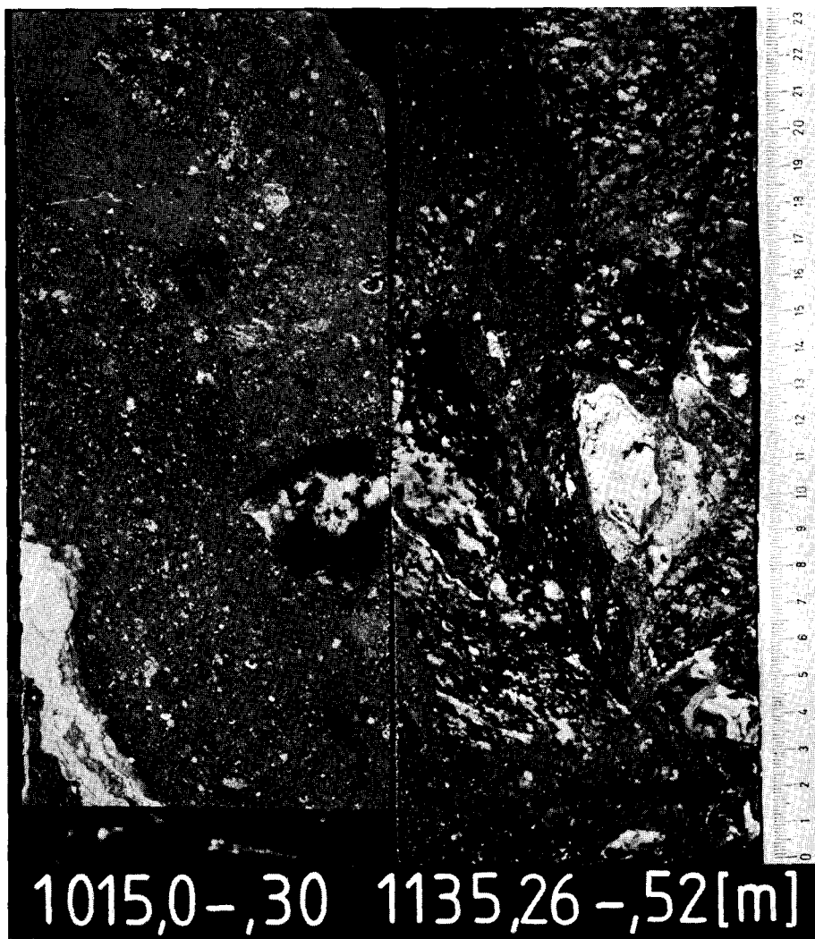
Fig. 7. Sections of dike breccias from the drill core of Nördlingen 1973. The vein-like intrusion into the biotite gneiss country rock is best visible in the right photograph. Lower left corner: brecciated fluorite dikelet. Scale = cm.
