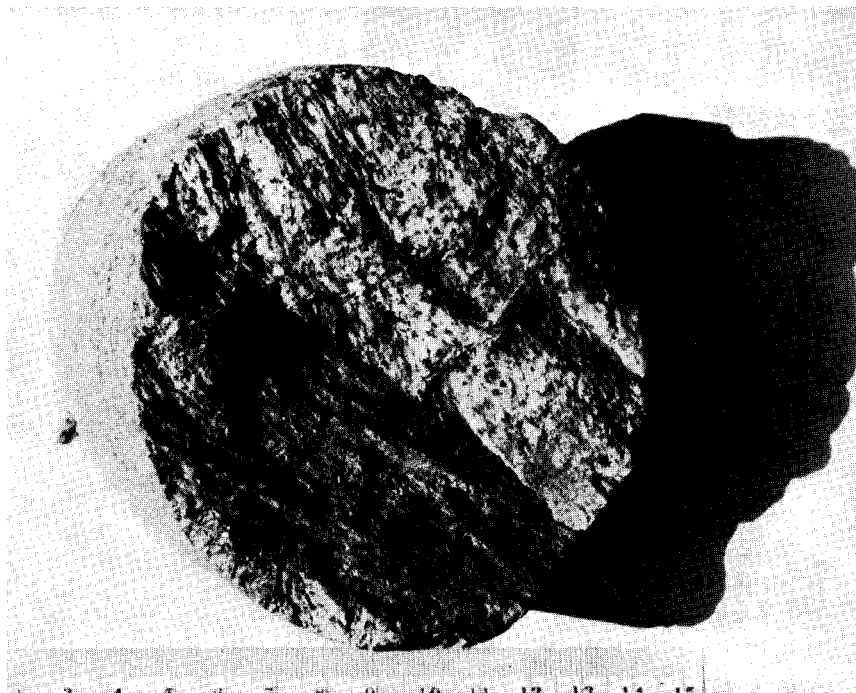
Fig. 4. Photograph of a section of drill core of chloritized granite from depth 605 m, showing a group of shatter cones with acute apices. Diameter of core 10 cm.
