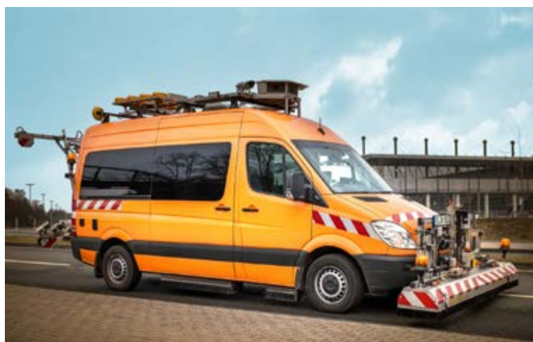
Multifunctional measurement system for assessing the surface condition of carriageways
